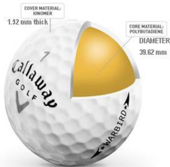
Figure 1 - A typical two-piece ball showing materials and dimensions. The cover is relatively thick and hard (about 70D). Many 'budget', 'value' or distance balls are like this. Picture produced with permission of Callaway Golf.
