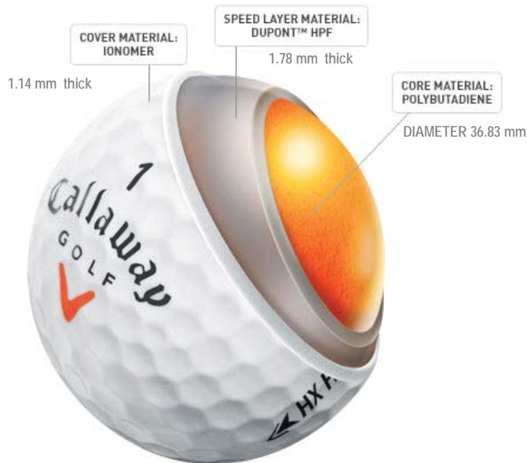
Figure 2 - A three-piece ball showing construction materials and dimensions. The cover is thinner and softer (about 60D) than that of the two-piece ball in Fig 1. Manufacturers whose top-of-the-range ball is three-piece have even softer and thinner cover – more like that of ball in Figure 3. Picture produced with permission of Callaway Golf.
