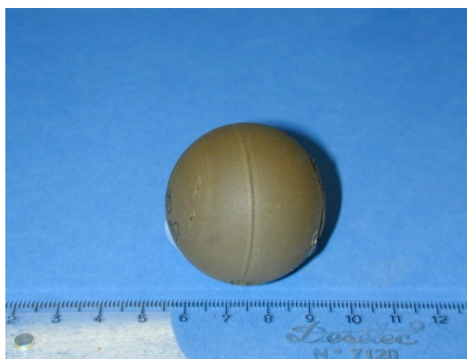
Figure 5 - Compression moulded rubber core showing seam running vertically.
